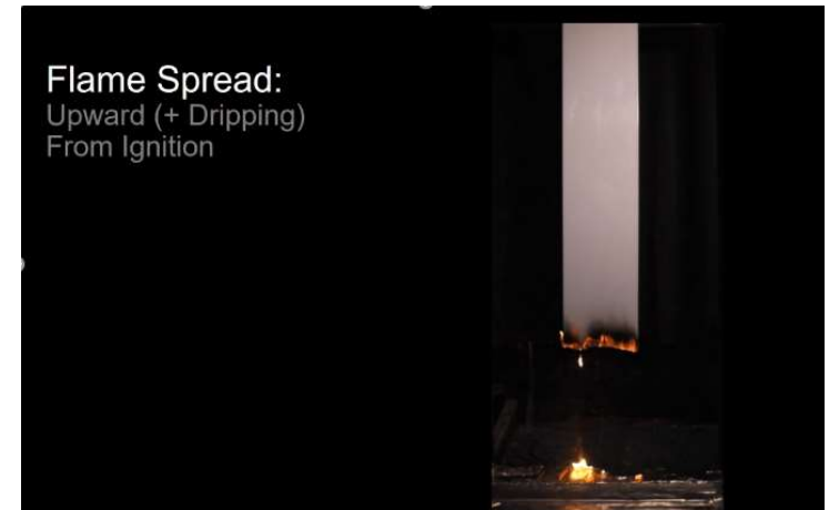
Vertical fire spread (upward and downward)
